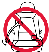
Lap belts with a sewn-in latch plate that have a retractor that locks only in case of a sudden stop.
