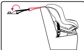
2. Pull the loose end of the webbing to remove slack from the tether.
