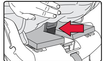
2. Remove the buckle strap by turning the buckle retainer sideways and routing it out of the front buckle slot in the child seat.
