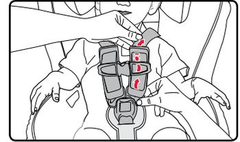
9. Pull the harness adjuster strap to tighten the harness.
