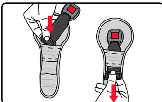
2. Route the belly pad and buckle retainer through buckle slot in the cover.
