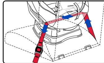
6. Push down on the middle of the child seat while pulling the vehicle belt to remove all slack.
