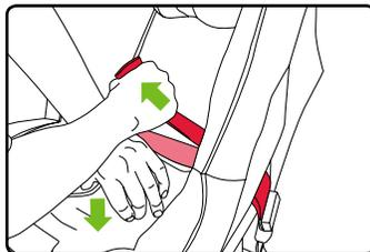
7. Attach the tether to a designated anchor (see vehicle owner's manual) and remove slack (see page 28). Wrap excess webbing in the elastic strap and store in tether storage pouch.
