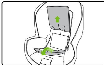
5. Route the vehicle seat belt through the forward-facing belt slots, ensuring the vehicle belt is not twisted, then buckle.
