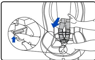
2. Recline the unoccupied child seat to position 3 and place rear-facing on the vehicle seat (see page 24). Ensure that no more than 3 in. (7.6 cm) of the base hangs over the edge of the vehicle seat.
