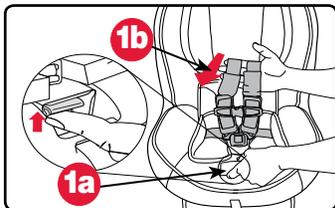
2. Squeeze the harness height adjuster, slide the harness into the desired position and release.
