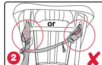
**IMPORTANT:** Discontinue use of child seat if it has been involved in a moderate or severe crash, regardless of whether the loops have pulled through the back side of the shell and the colored stitching has been ripped.
