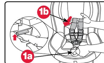
2. From the back of the seat, unhook the harness straps from the yoke.
