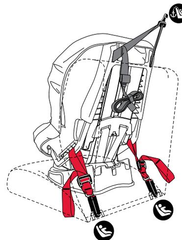
Do not install forward-facing with the lower anchors for a child weighing more than 50 lbs (22.7 kg).
