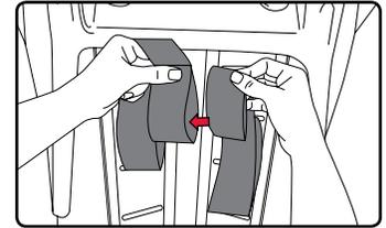
9. Hook the harness straps onto the yoke. Ensure that the harness straps are not twisted and that the ends of the harness straps are securely attached to the yoke.
