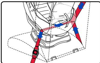
7. Push down into the middle of the child seating area with moderate force while removing all slack from the bottom (lap) part of the vehicle belt and close the lock-off (see page 24).
