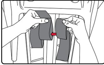
9. Hook the harness straps onto the yoke. Ensure that the harness straps are not twisted and that the ends of the harness straps are securely attached to the yoke.
