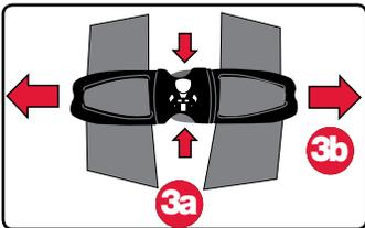
4. Release the buckle and attach the harness straps to the harness holders.
