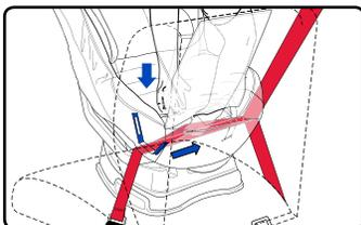
8. Push down into the middle of the child seating area with moderate force while pulling the top (shoulder) part of the belt between the belt slots to remove any remaining slack through the lock-off.
