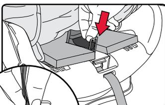
4. Turn the buckle retainer sideways and route it through the front buckle slot and then into the desired buckle position (see page 22).
