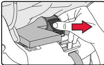
4. Pull the end of the belly pad and buckle retainer out of the slot in the cover to remove.
