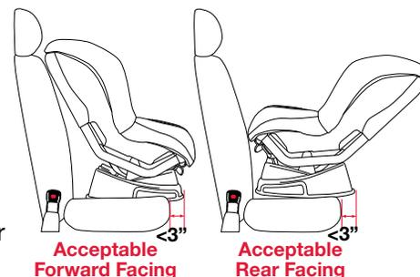
Some vehicle seats do not allow enough of the child seat base to contact the vehicle seat. If this is the case for a forward-facing installation, adjust the seat to the upright position. For a rear-facing installation, choose another seating position. Not doing so could cause the child seat to not perform as intended.
