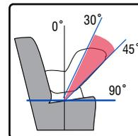
Use the line as a guide to achieve the proper recline angle for rear-facing installations. The line will be parallel to the ground when the child seat angle is at the center of the acceptable angle range (37.5°). If necessary, the proper recline angle can be achieved by placing a rolled towel or pool noodle in the vehicle seat bight.
