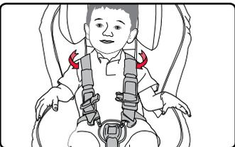
7. Fasten the harness buckle. Proper connection is confirmed with a click after inserting each buckle tongue.
