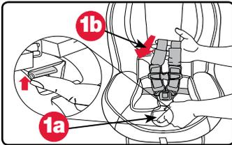
2. From the back of the seat, unhook the harness straps from the yoke.
