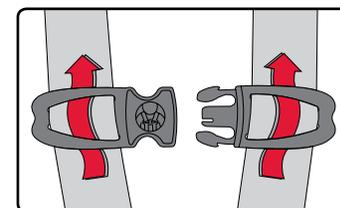
5. Reroute the harness strap back through the chest clip, ensuring that the harness strap is not twisted.
