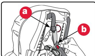
**NOTE:** The tether carry clip is only for use when you wish to carry the child seat between locations. When used as a carry strap, tighten until the strap is comfortable to carry. **Do not install the child seat with the tether attached to the carry clip.**
