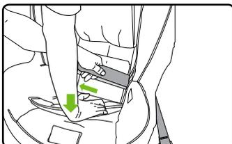
8. Push down into the middle of the child seating area with moderate force while pulling the top (shoulder) part of the belt between the belt slots to remove any remaining slack through the lock-off.
