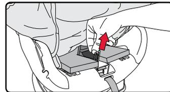
2. Route the belly pad and buckle through the desired slot in the cover.
