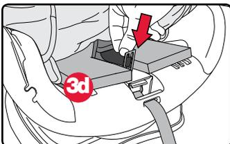
3. Attach the plastic hooks to the bottom edge of the child seat.
