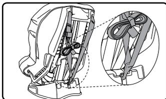
Secure the excess tether webbing in the elastic strap during use. Store the tether in the storage pouch when not in use. Always ensure any excess webbing is contained within your vehicle.
