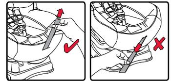
✓ Pull the harness adjuster strap up and away from the child seat to tighten.
