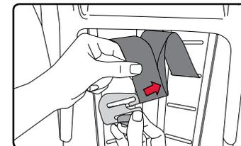
3. Pull one harness strap through the harness slot to the front of the seat.
