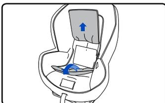
4. Open the blue lock-off closest to where the vehicle belt will be buckled.
