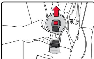
5. Turn the buckle retainer sideways and route the buckle assembly out of the belly pad.
