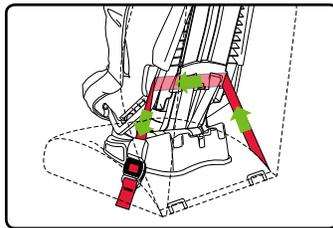
6. Push down on the middle of the child seat while pulling the vehicle belt to remove all slack.
