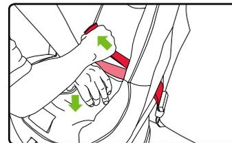
9. Attach the tether to a designated anchor (see vehicle owner's manual) and remove all slack (see page 28). Wrap excess webbing in the elastic strap and store in tether storage pouch.
