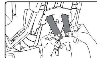
7. Route the harness straps through the seat to the back. Ensure that the harness straps pass through the harness adjuster.
