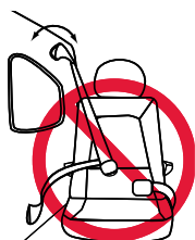
Lap-shoulder belts with top or bottom anchor points on the vehicle door.
