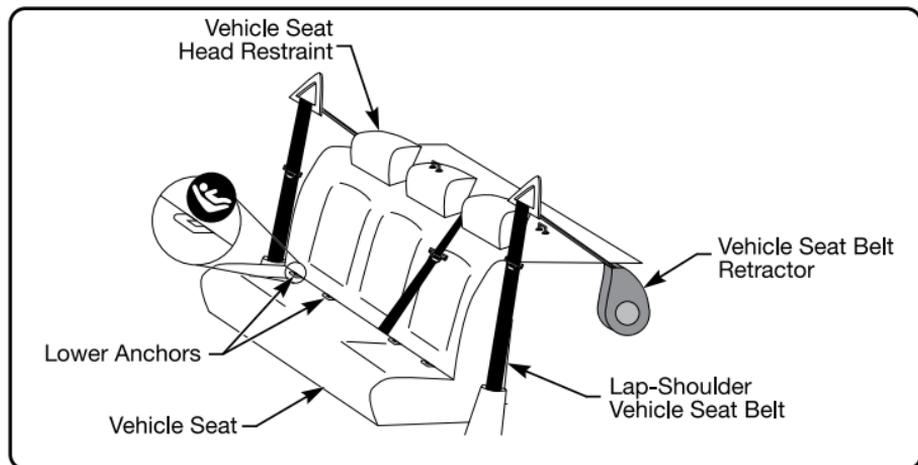
Check your vehicle owner's manual to learn if it is equipped with lower anchors, the maximum weight rating and information on the lower anchor locations and designated seating positions available for use with this child seat.
