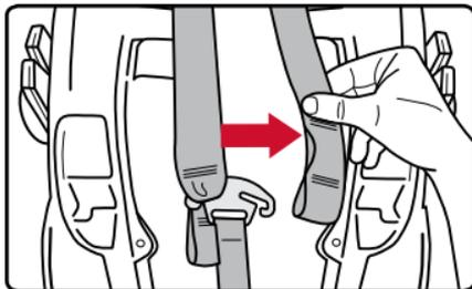
3. From the front of the seat, pull the harness strap through the cover and head pad.
