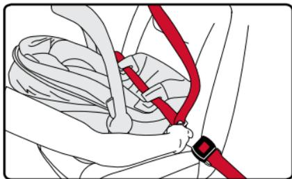
4. Verify that the vehicle belt is not twisted and buckle. Lock your vehicle seat belt system as instructed by your vehicle owner's manual.
