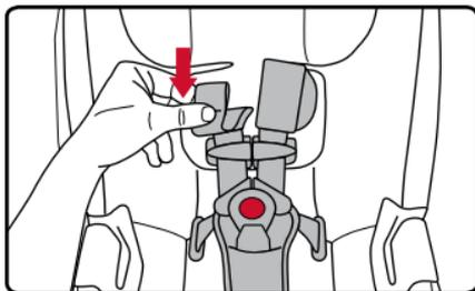
4. Ensure that the harness strap is not twisted and rethread the harness strap through the head pad and then through the appropriate harness height slot in the cover and shell.
