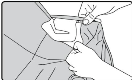
7. Slide each side of the harness, with the buckle tongue and chest clip, through the cover and pull the cover off of the shell.
