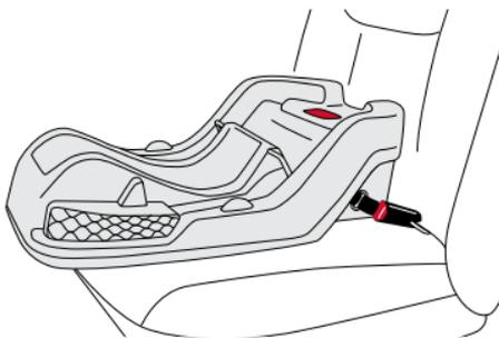
Base Installation with Lower Anchors
