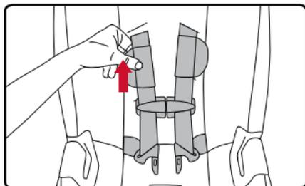
2. Loosen the harness by pressing down the harness adjuster lever while pulling both harness straps forward.
