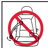
5 Lap belts that have a retractor that locks only in case of a sudden stop (emergency locking retractor- or ELR).
