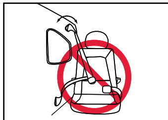
1 Vehicle belts with top or bottom anchor points on the vehicle door.
