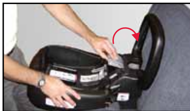
Base Installation with Lap-Shoulder belt
