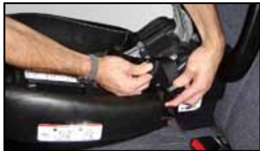
Base Installation with LATCH
