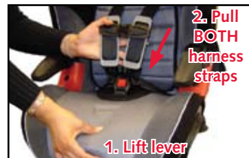
1 Loosen the harness by lifting the harness adjuster release lever located on the front of the child seat while pulling BOTH harness straps forward.
