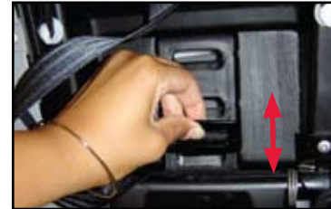
3 Slide the buckle retainer back into place to hold it against the child seat shell.
