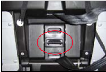
1 Locate the metal buckle strap retainer on the bottom of the child seat.
