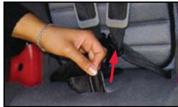
6 Pull the buckle retainer through the slots in the child seat shell and cover to the top of the child seat.
