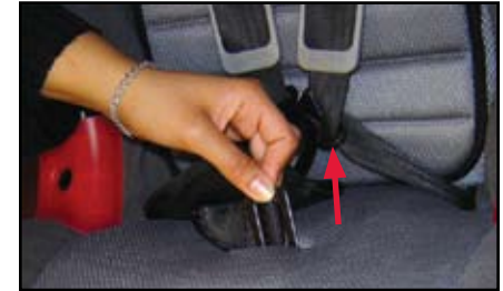
5 Pull the retainer through the slots in the child seat shell and cover to the top of the child seat.
