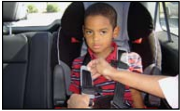
5 Place the child in the child seat and position the harness straps around the child.
