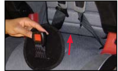
4 Pull the buckle away from the child seat until tight. Verify that the buckle retainer lies flat against the child seat shell.
