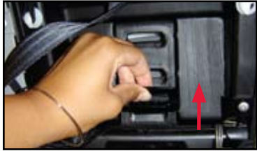
11 Slide the buckle retainer up or down to release it from the child seat shell.
