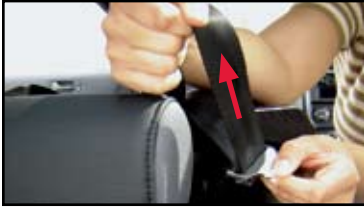
3 Tilt the tether adjuster tab and pull to fully extend the tether.
