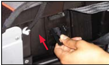
5 Turn and push the buckle retainer so that the short side will pass through the slot in the child seat shell
