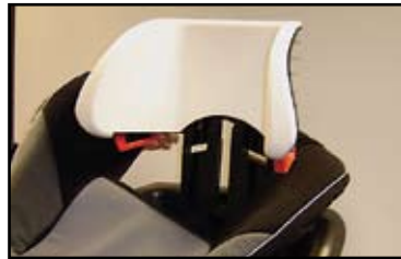
16 Route the cover around the head restraint and remove the entire cover from the child seat shell.
