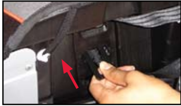
13 Turn and push the buckle retainer so that the short side will pass through the slot in the child seat shell.
