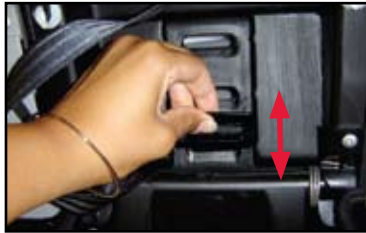
3 Slide the buckle retainer up or down to release it from the child seat shell.
