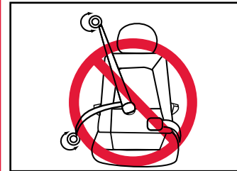
4 Lap-shoulder belts that have a separate retractor each for the lap and shoulder parts.
