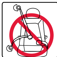
Lap-shoulder belts that have a separate retractor each for the lap section and shoulder section.
