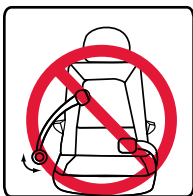
Lap belts with a sewn-in latch plate that have a retractor that locks only in case of a sudden stop.
