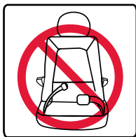
Lap belts forward of the vehicle seat bight.
