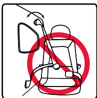
Lap-shoulder belts with top or bottom anchor points on the vehicle door.
